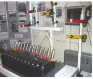
The miniature lever frame and signals in the locking room. 6 of the levers operate the signals and demonstrate the principals of interlocking to visitors.
