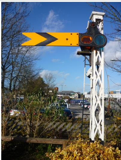
Above: the lattice post now carries a distant signal arm worked from the ground frame.
