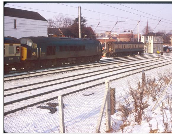
'Peak' Class number 45 119 passing on a down express on a snowy day some time post 1982. The regular parcels van sits in the siding alongside the box and a temporary 55mph speed restriction board sits in between the fast and slow lines.
