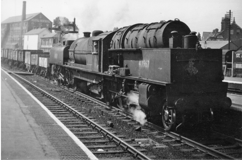
On 31 July 1955 Beyer-Garratt 2-6-0+0-6-2T 47967 trundles through St Albans City Station with a northbound train of empty coal wagons. The Signal Box and Heath and Heather building are in the background. The locomotive was built for the LMS in 1930 and spent most of its life shedded at Toton. The rotating bunker was fitted in the mid 30s. It was withdrawn from Hasland Shed in December 1957.
